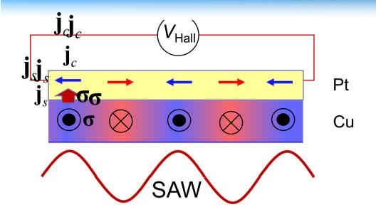
Inverse  $\mathbf{j}_{c} = \theta_{\text{ISHE}} \left( \frac{2e}{\hbar} \right) \mathbf{j}_{s} \times \boldsymbol{\sigma}_{\boldsymbol{\sigma}}$ Hall yolt Non-uniform spin current is compensated...
