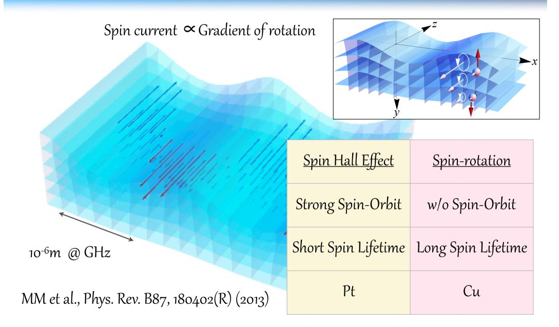
Cu can be utilized for spin-current source!  $\rightarrow$  Rare metal free spintronics
