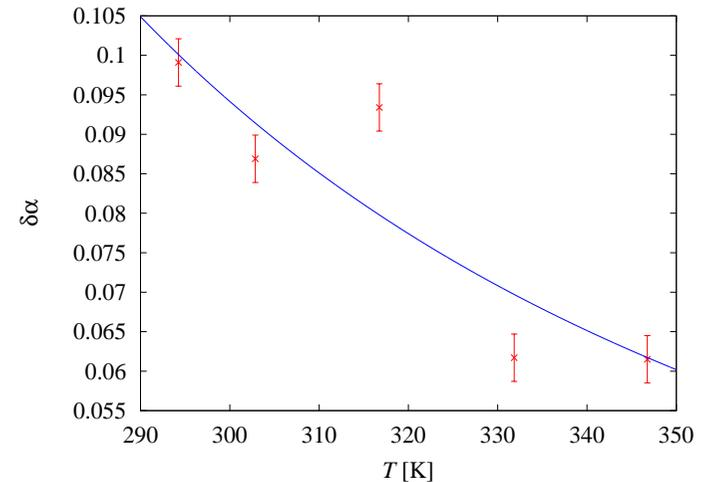
Oil surface fluctuations:  $T = 21, 30, 59, 74$  °C. Good agreement, slight deviation at high frequencies. Mismatch larger for smaller  $T$ .
